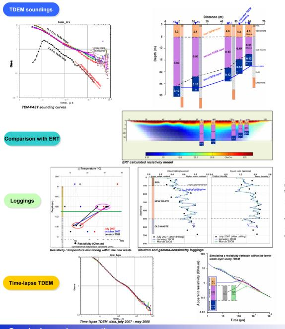
> TDEM response free from inductive effect (metallic conductors) thanks to high conductive response from waste.
